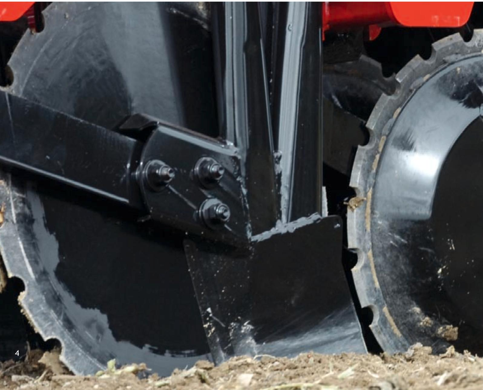
The separately weighed support wheels distribute the machine's weight out evenly throughout the seeding width. The packer wheels follow the contours of the field closely, ensuring that the seed has good contact with the soil and retaining excellent starting moisture.
